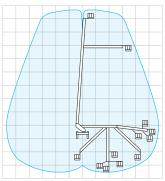
The 48m Palfinger's full range of movement can be seen in the graph
